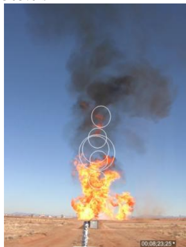
Figure 97 LNG Test 1 180° spoke HD camera stills with NV radiometer overlays.
