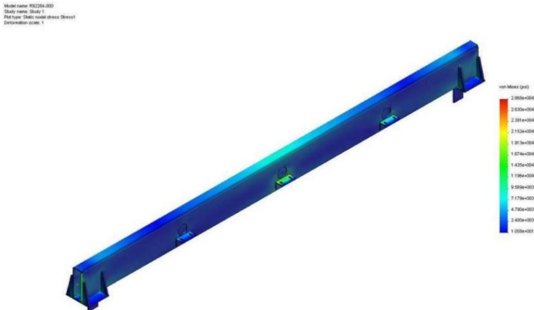
Figure 36 FEA stress analysis of the A-frame.
