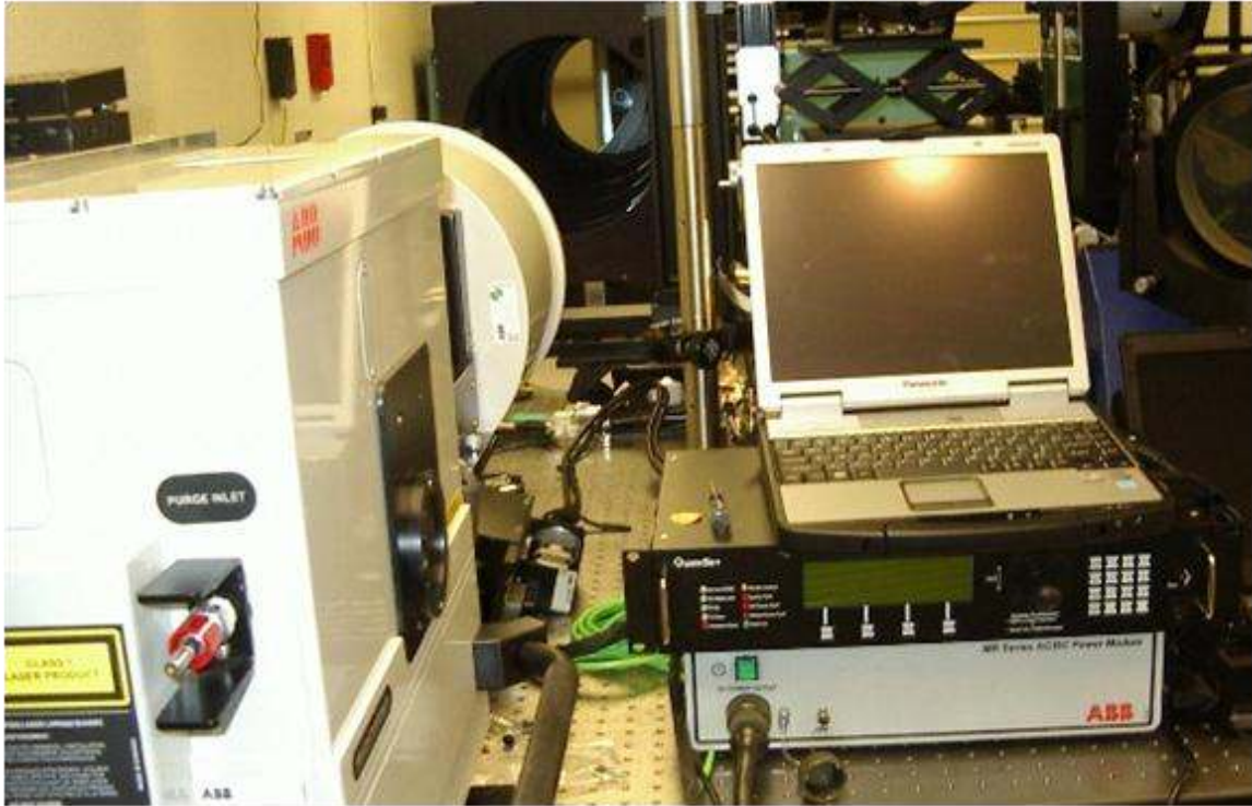
Figure 70 FTIR with narrow telescope aligned with collimator.
