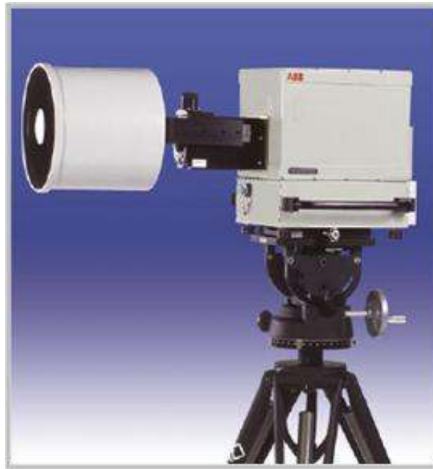
Figure 66 ABB - Bomem FTIR radiometer.
