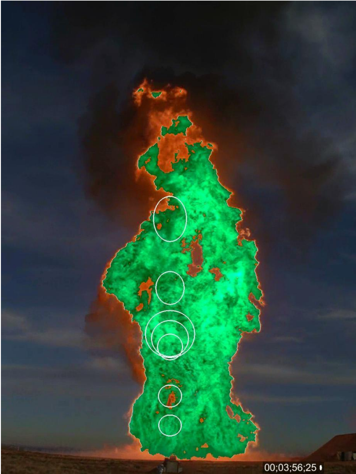
Figure 230 South spoke camera view with NV radiometer field of view overlay (t=233.5s).
