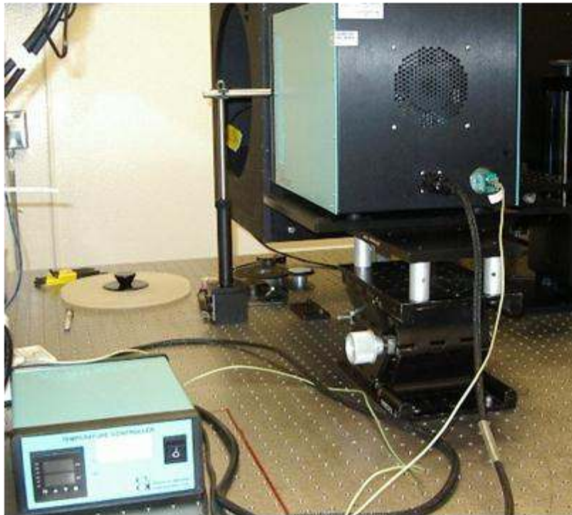
Figure 69 Blackbody source at input of the collimator.
