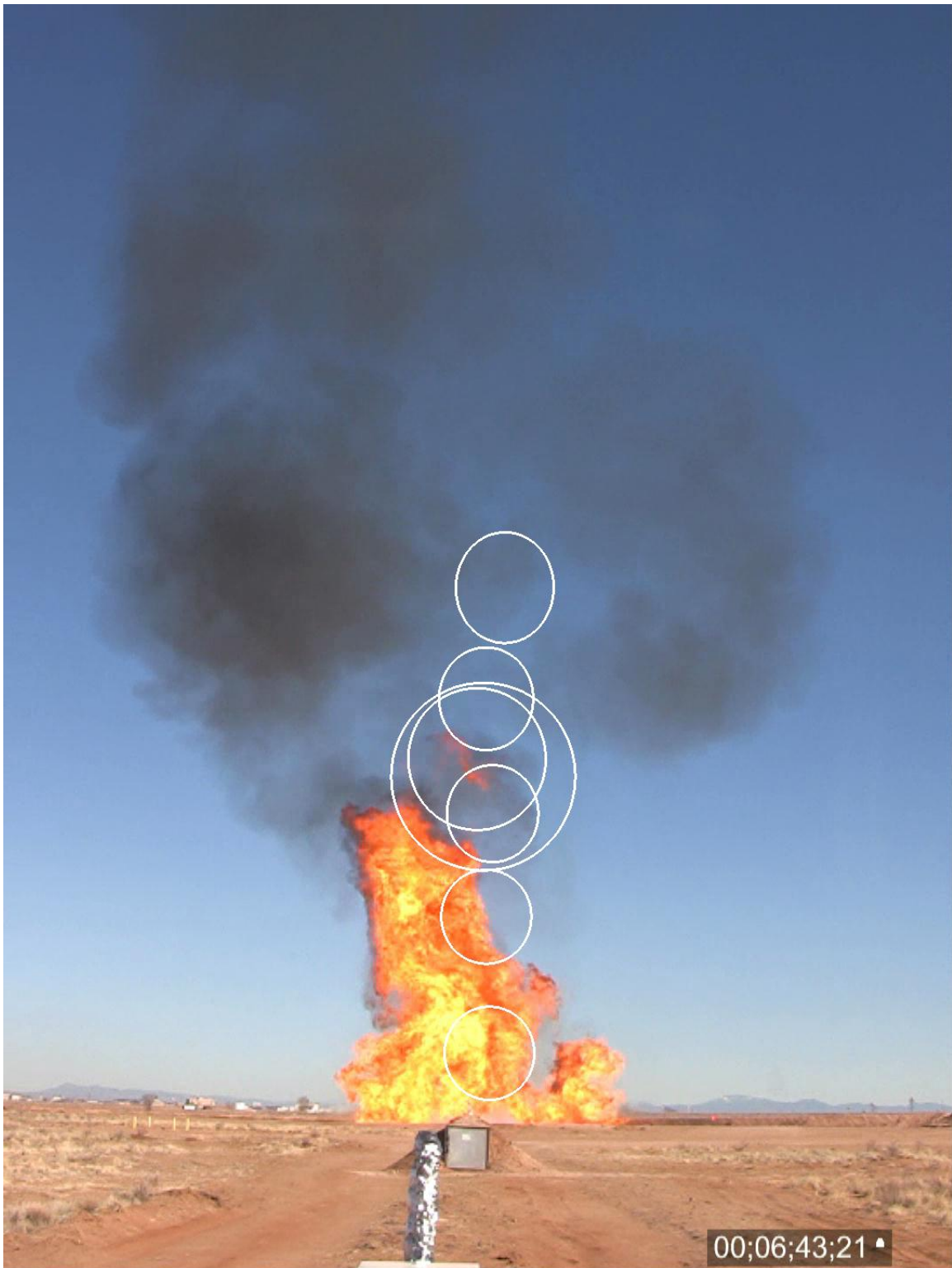
Figure 137 South spoke camera view with NV radiometer field of view overlay (t = 403.7 s).
