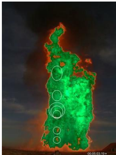
Figure 195 LNG Test 2 180° spoke HD camera stills with NV radiometer overlays.
