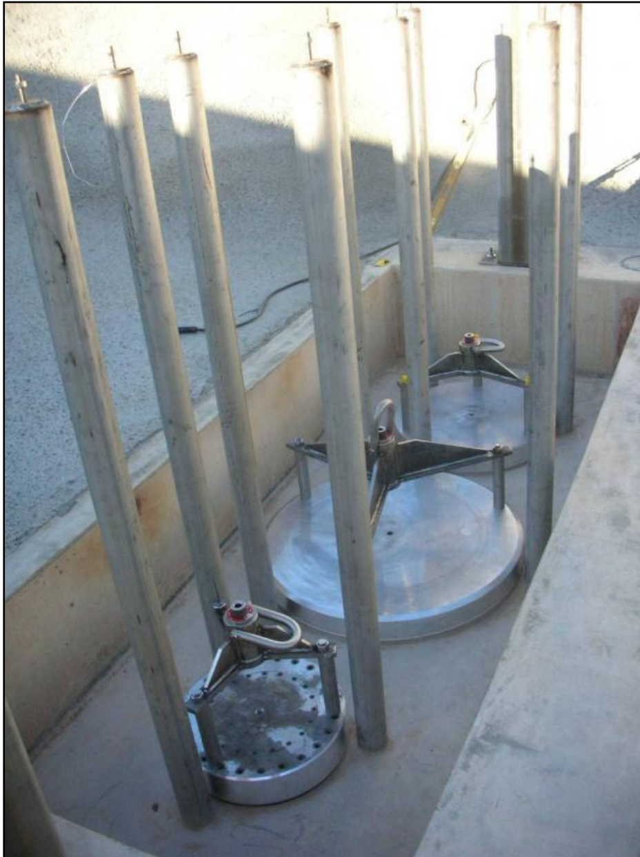
Figure 34 LNG plugs with lift fixtures and swivels.
