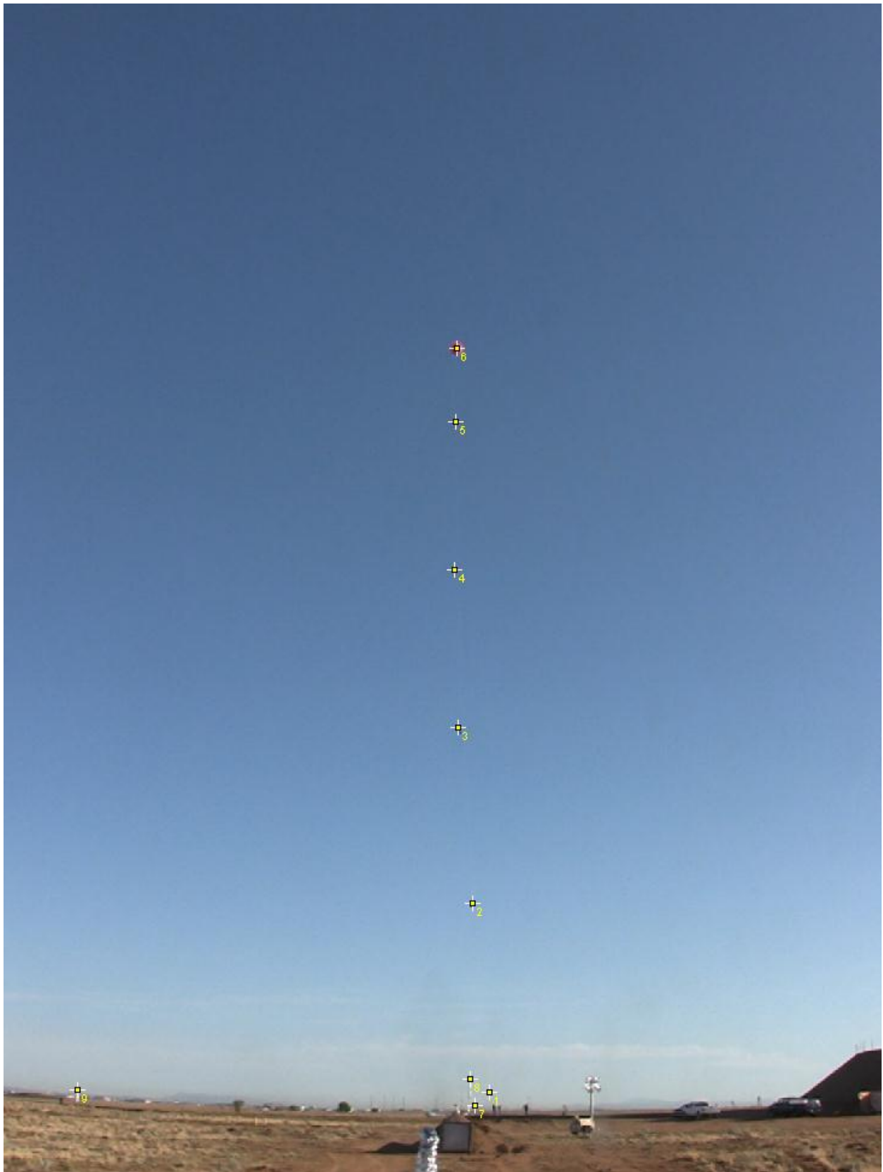
Figure 4 Calibration image showing the extracted calibration points
