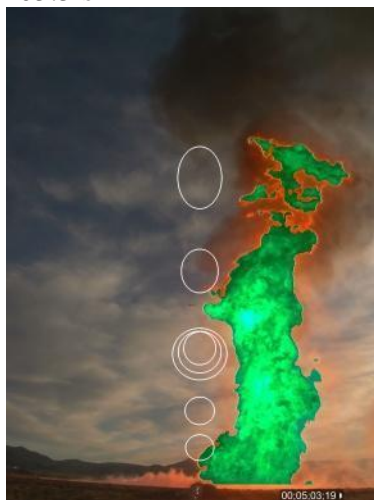
Figure 196 LNG Test 2 270° spoke HD camera stills with NV radiometer overlays.
