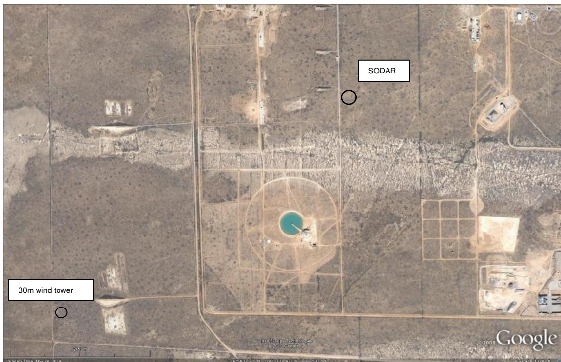
Figure 76 Site locations of meteorological support instruments.
