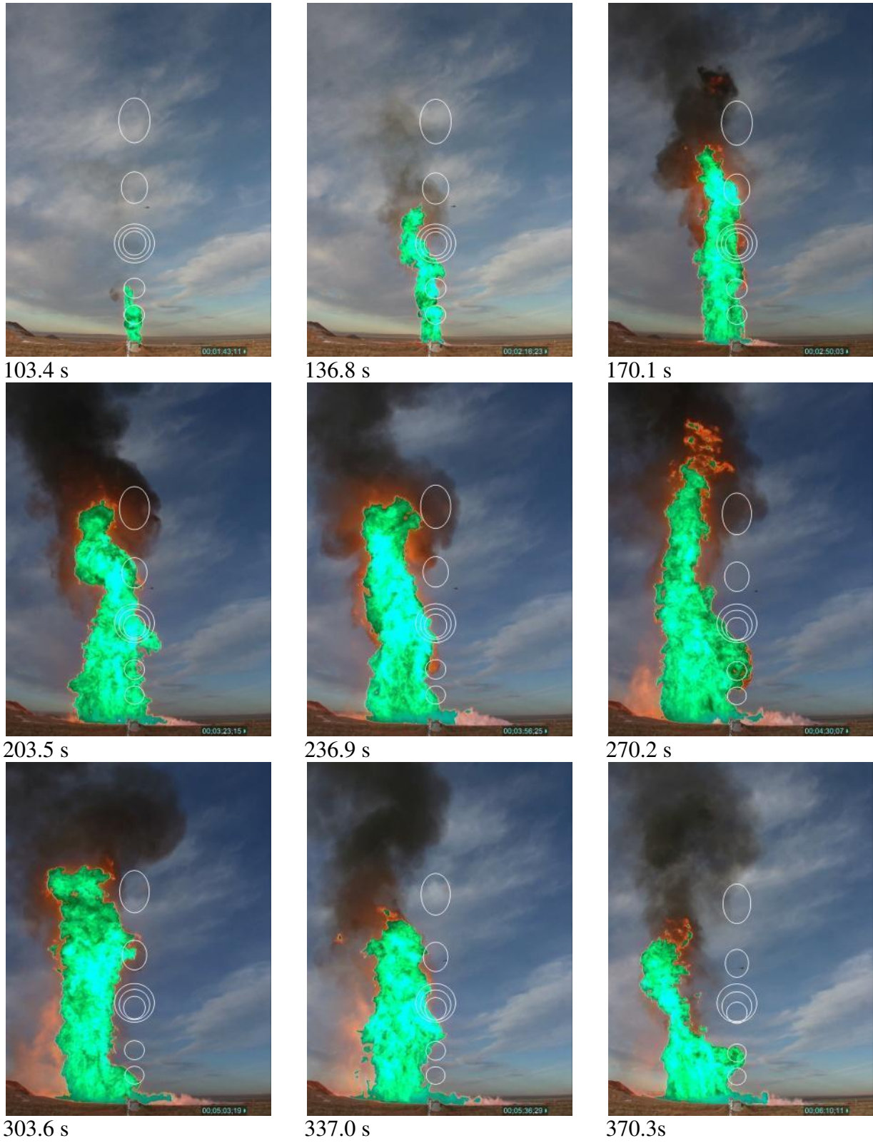
Figure 194 LNG Test 2 90° spoke HD camera stills with NV radiometer overlays.
