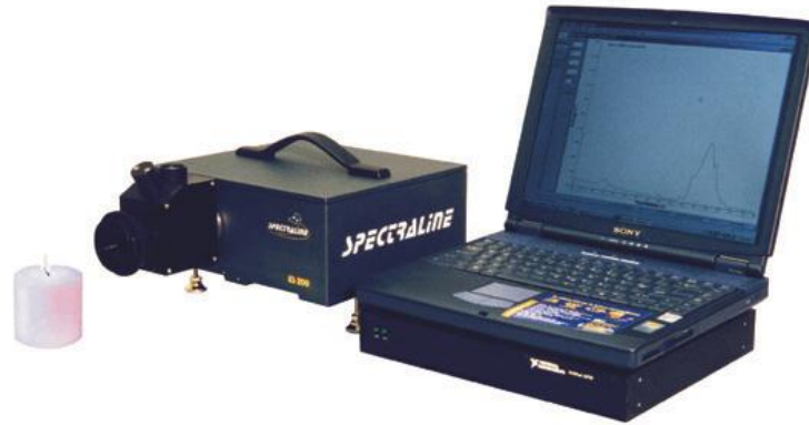
Figure 60 Spectraline ES200, laptop, and data acquisition system
