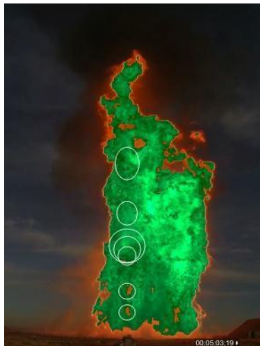
Figure 195 LNG Test 2 180° spoke HD camera stills with NV radiometer overlays.
