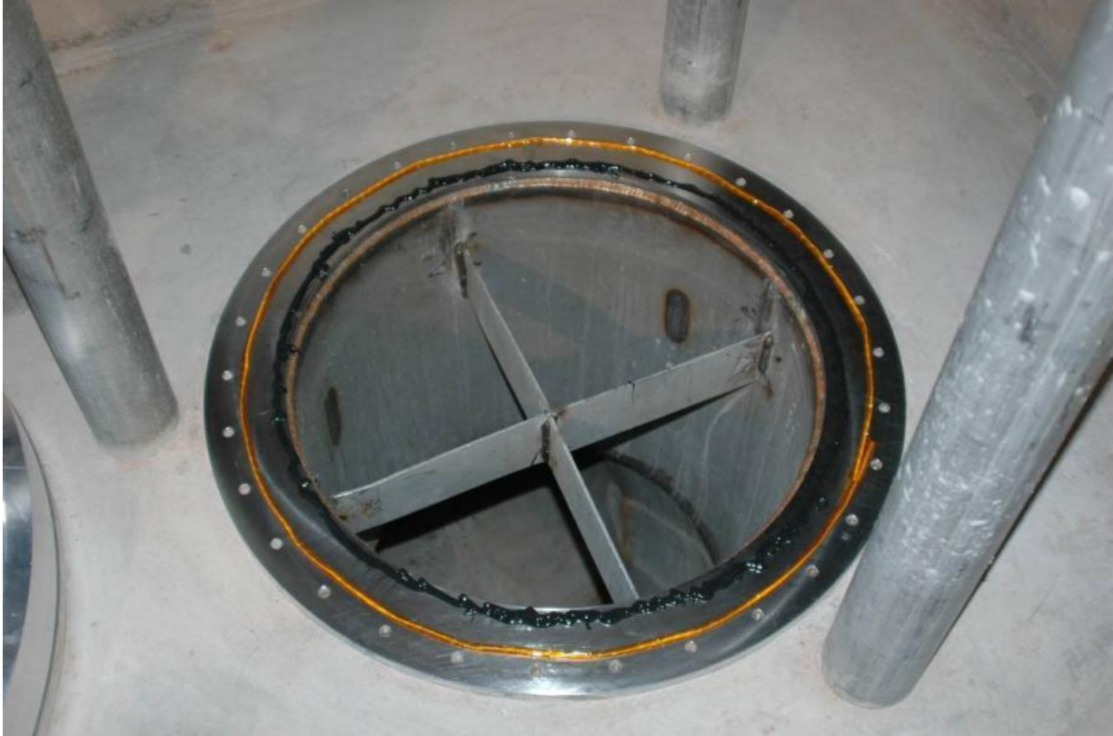
Figure 84 Formed gaskets on the 36 inch discharge pipe flange in Test 1.
