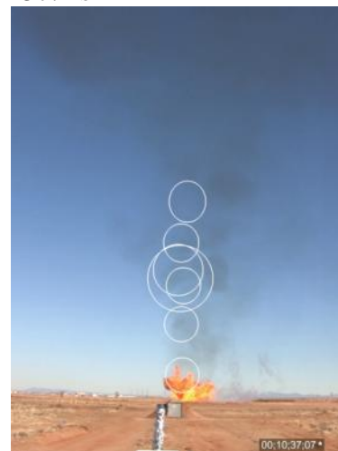
Figure 97 LNG Test 1 180° spoke HD camera stills with NV radiometer overlays.
