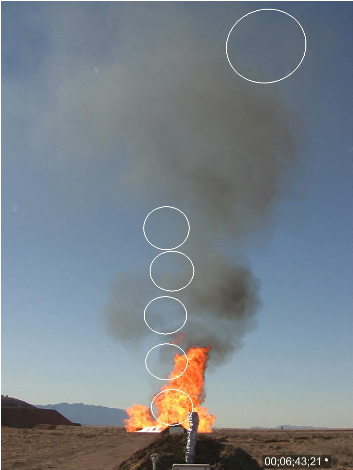
Figure 134 North spoke camera view with NV radiometer field of view overlay (t=403.7 s).
