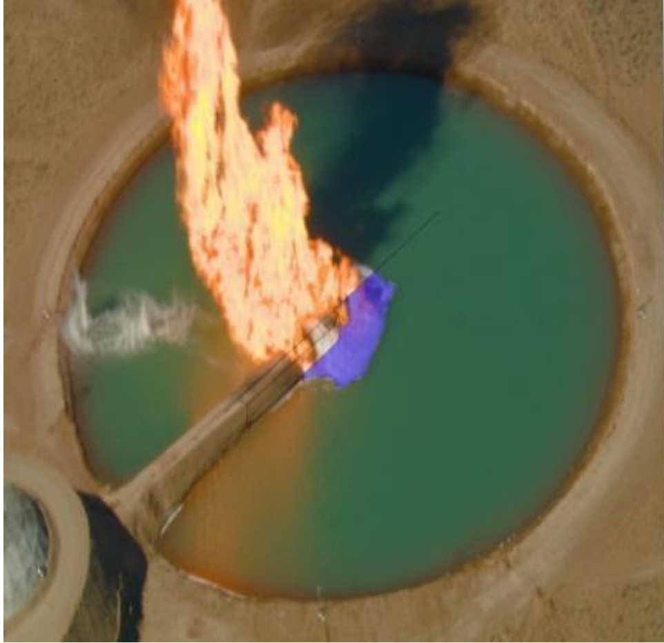
Figure 91 Test 1 aerial view at 420 s used to determine spreading pool area.
