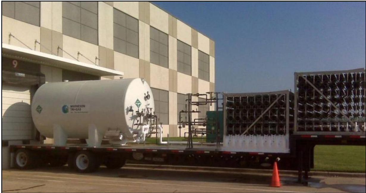
Figure 41 Nitrogen gas source trailer.
