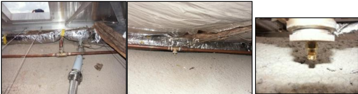
Figure 164 Fabrication of LN 2 spray ring with nozzles internal to reservoir.
