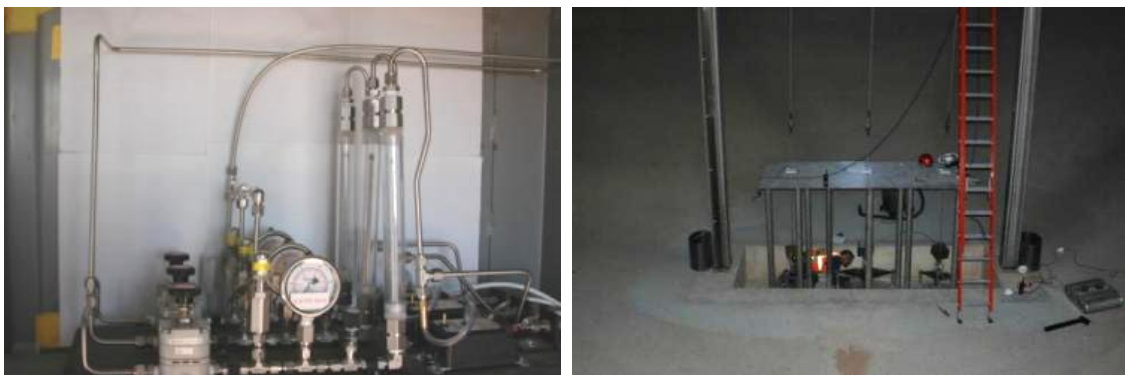
Figure 58 Diptube instrument setup and tube exit locations near the reservoir floor.
