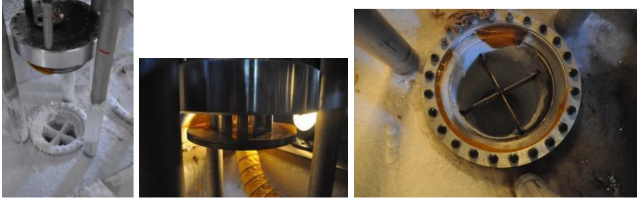
Figure 165 The 15 inch plug after the October LN 2 cool down and leak test.
