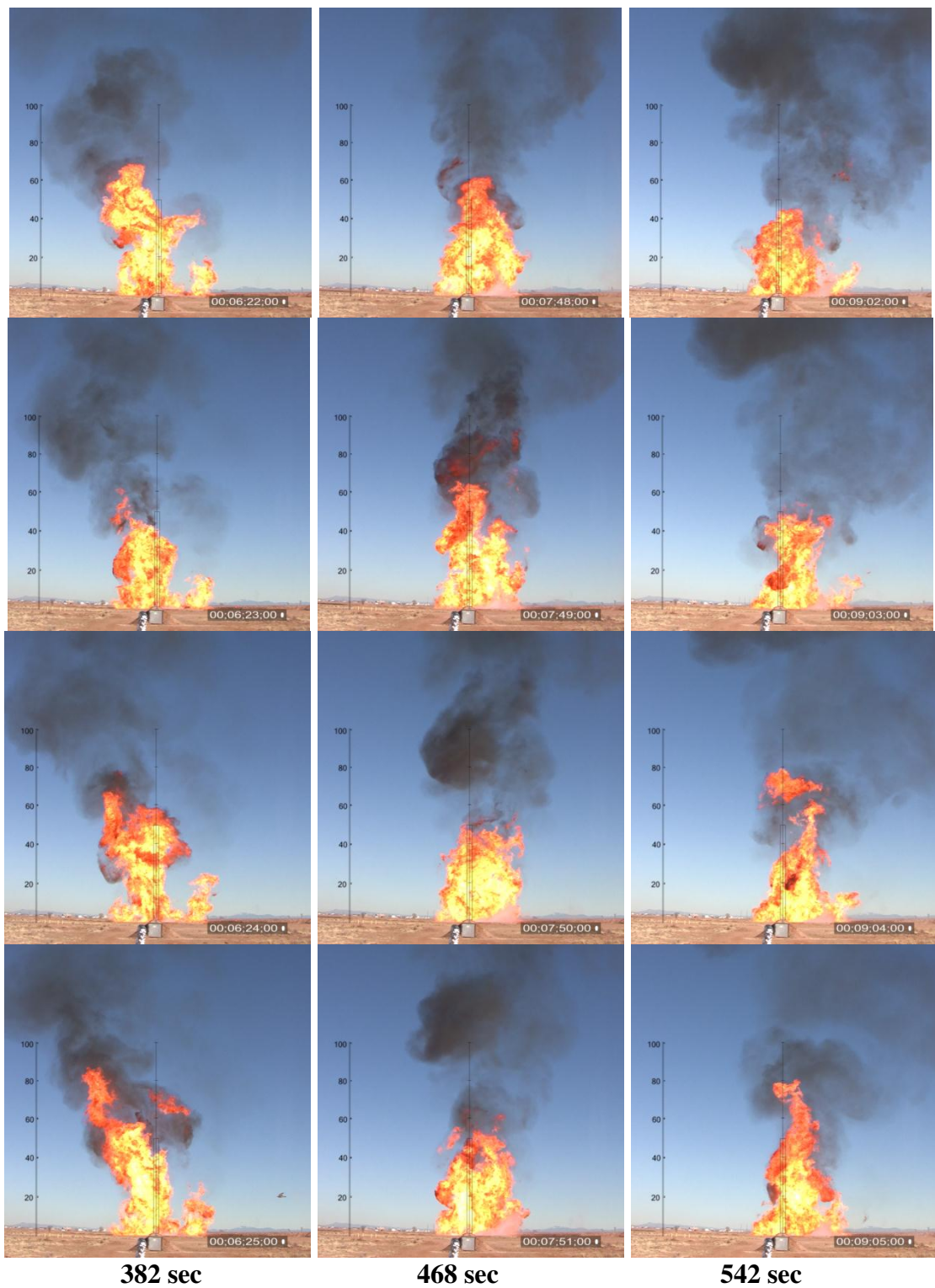
Figure 141 LNG Test 1 images with the South spoke spectrometer FOV overlay.
