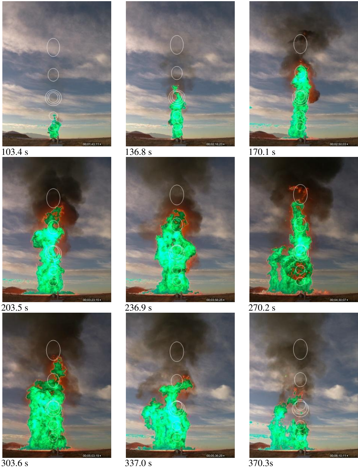
Figure 193 LNG Test 2 0° spoke HD camera stills with NV radiometer overlays.
