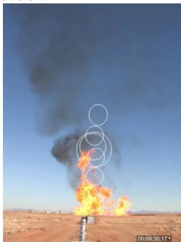
Figure 97 LNG Test 1 180° spoke HD camera stills with NV radiometer overlays.
