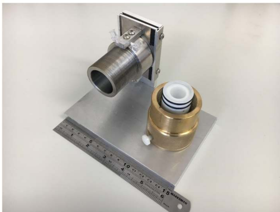
Figure 11. Photograph of the variable path length optical cell used to record the effect of solute concentration on the absorption and fluorescence spectral properties of TIPS-P in toluene. A screw barrel allows easy variation of the path length while the double seal prevents leakage of solution. The set-up fits comfortably into a range of spectrophotometers. Calibration of the path length is made by reference to standard solutions and/or birefringence effects.
