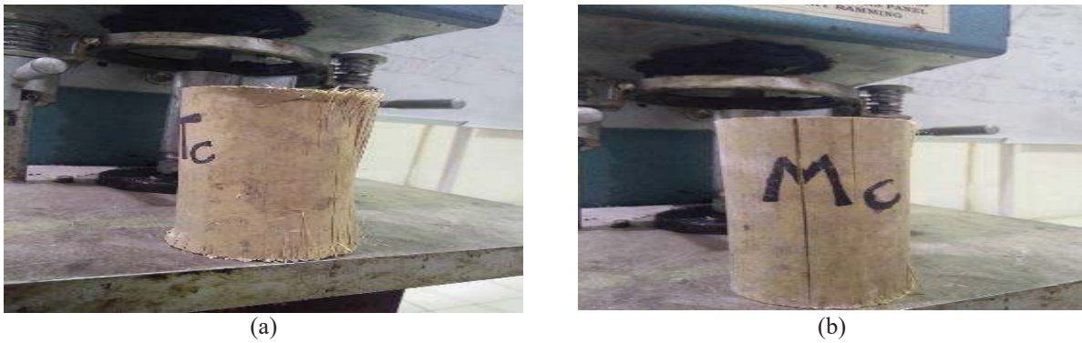
FIGURE 4. Compression strength test (a) End bearing failure mode (b) Splitting failure mode
