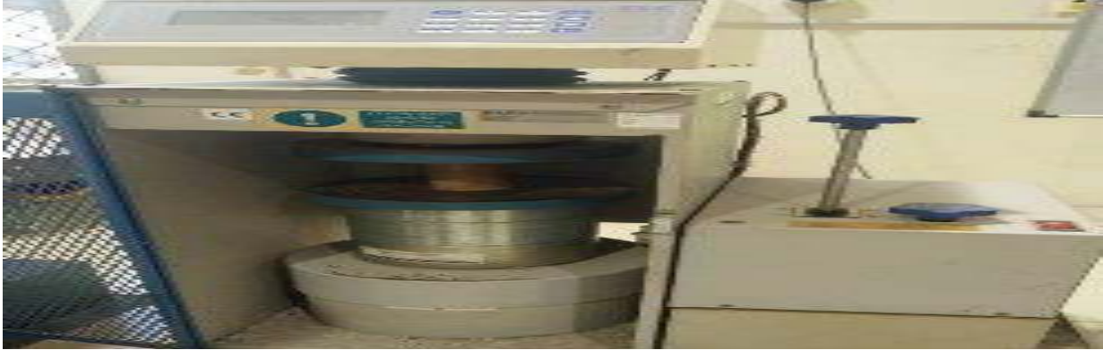
FIGURE 1. Setup for compression test
