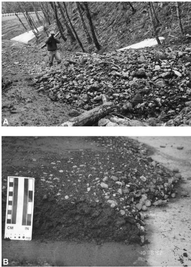
Figure 12. Photographs of snouts of debris flow deposits, which show concentrations of coarse clasts and bluntly tapered margin morphology. (a) Lobe of a small ( \sim 1000 \text{ m}^3 ) debris flow that partly crossed the scenic highway near Benson State Park, Oregon, February 7, 1996. (b) Vertical cross section through a marginal lobe of an experimental debris flow at the USGS debris flow flume, October 8, 1992.
