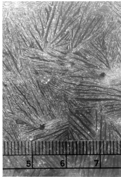
FIG. 12. The underside of the laboratory-grown sea ice showing the cellular solid/liquid structure of the interface and two clear brine-drainage channels. The c axes of the ice crystals are oriented principally horizontally, parallel to the plane of the page, displaying the columnar structure and permeability of natural sea ice. The large-scale is in cm. Adapted from Wettlaufer et al. , 1997.
