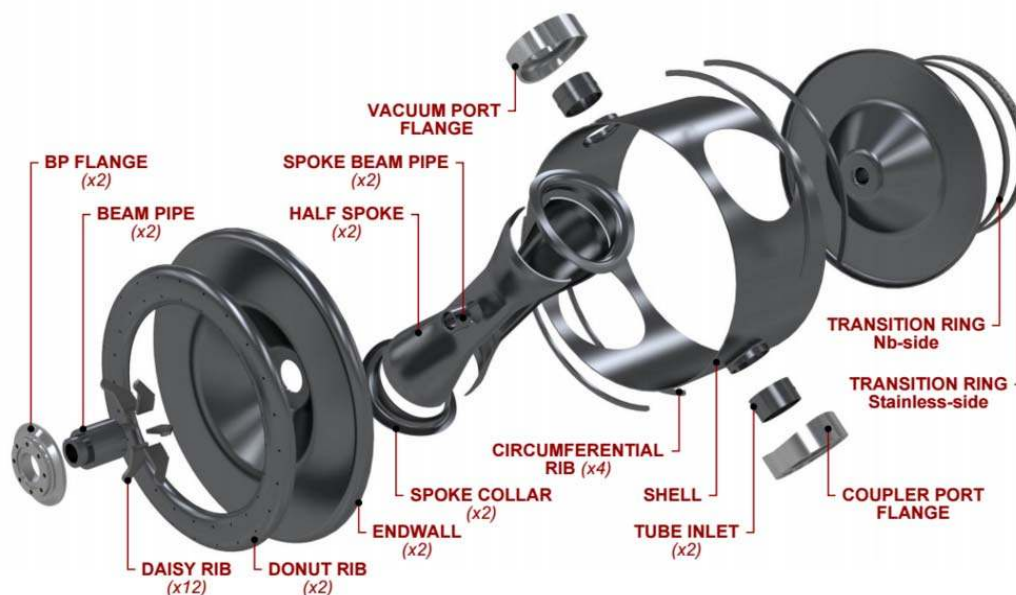
Figure 3.42: Exploded view of the bare niobium SSR1 cavity.
