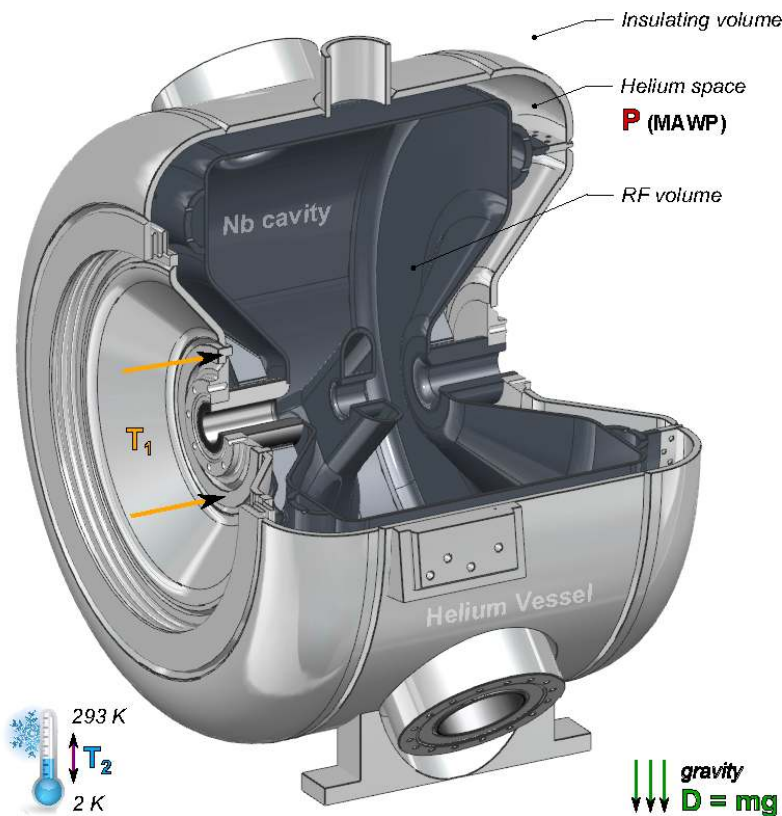
Figure 3.44: Cutaway view of jacketed SSR1 cavity with schematic loads applied. The pressure ( P ) is applied normal to the surfaces confining the helium space, the frequency tuning displacement ( T_1 ) is applied normal to the beam pipe (along the arrows), the gravitational force ( D ), and the cooldown ( T_2 ) applied to the entire system.
