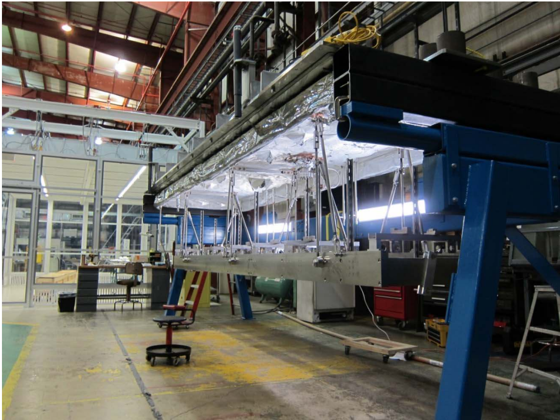
Figure 3.36: The titanium strong-back hung from the lid of the half-wave resonator lid. No cavities or solenoids are mounted on the strong-back.
