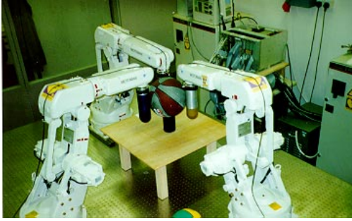
Figure 6: Three cylinder fingertips manipulating a ball
