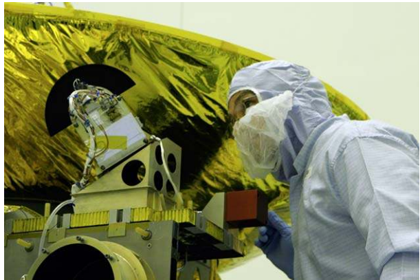
Fig. 1 PEPSSI mounted on the New Horizons spacecraft via its complex-angle bracket in the clean room at APL prior to being covered with its thermal blanket
