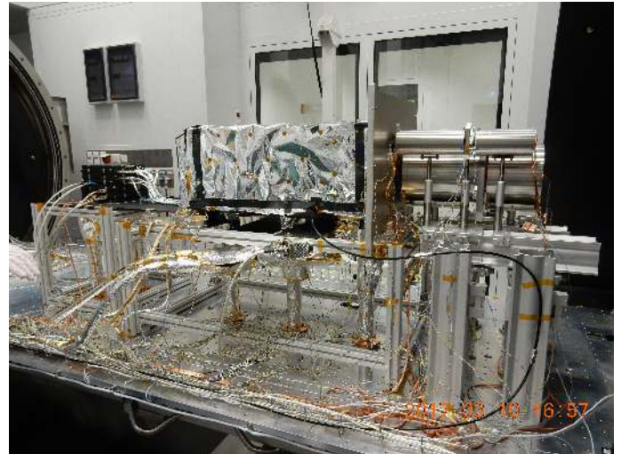
Fig. 28. SO/PHI Flight Model thermal test setup prior to insertion into the large thermal vacuum chamber at MPS.
