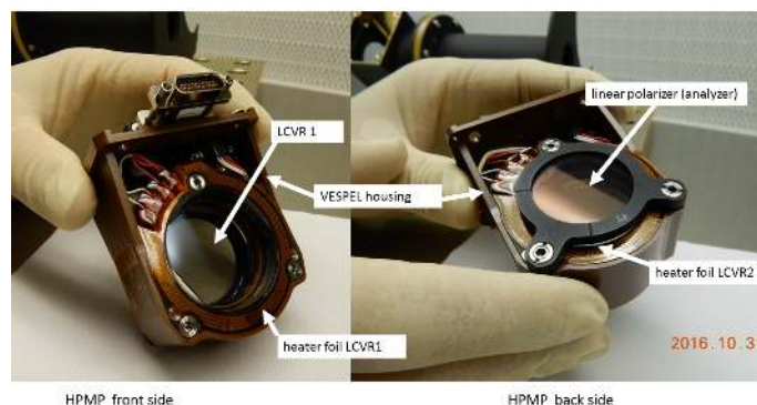
Fig. 17. Polarisation State Analyser of the HRT path.
