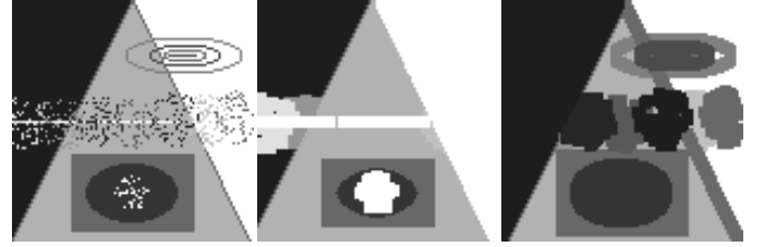
Figure 1. : Left Sample image of size 99 \times 99 . Centre: Dilation. Right: Erosion, with a 5 \times 5 flat filter.
