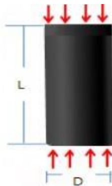
Fig. 2: Loading of specimens in the direct compression test.
