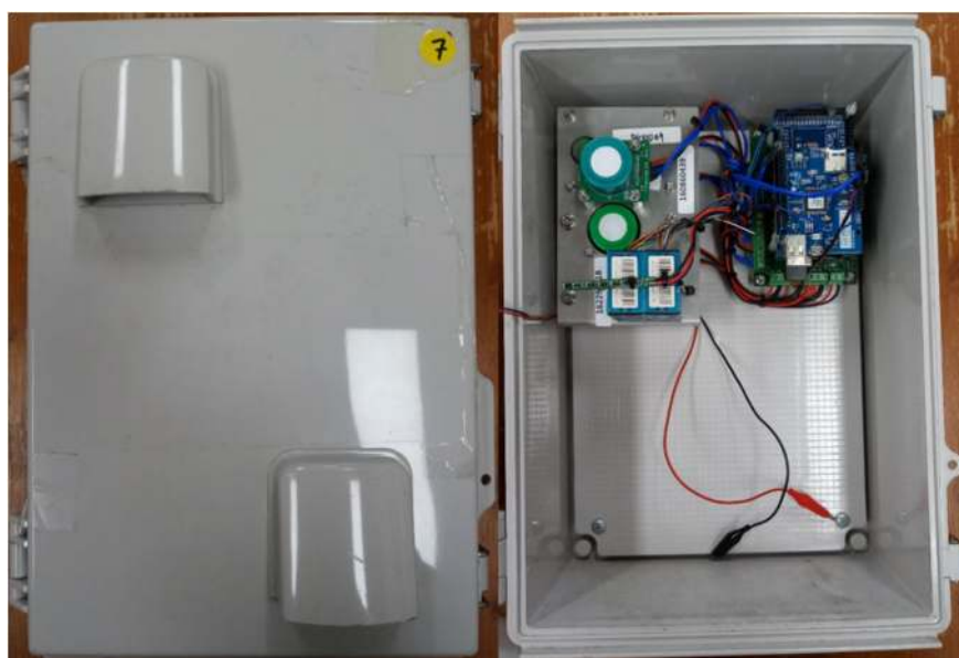
Fig. 1. Image of the sensor assembly. The space at the bottom holds the battery.
