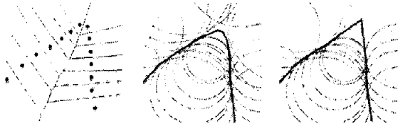
Figure 11. The inner poles of the samples near a sharp corner do not pass the 'skinyness' test. But just discarding the inner poles collapses the power crust at the corner. Discarding both poles of the badly-shaped Voronoi cells allows the power crust faces formed in nearby well-sampled regions to extend into the region of uncertainty and meet at a sharp corner.
