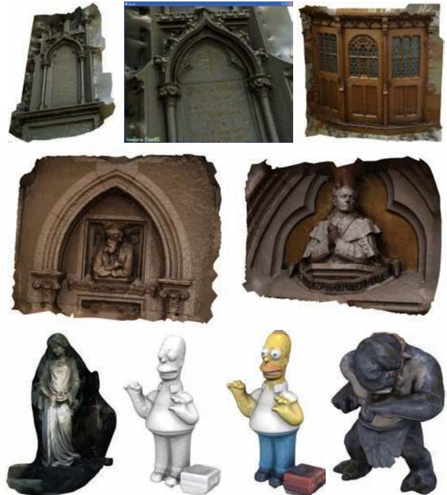
Figure 10: Models from the Herz-Jesu Church in Graz each reconstructed from 6-12 photos (6 MP) using the Epoch Webservice (KU Leuven) and the Meshlab software (CNR Pisa). Bottom: Water-tight models from the Poisson reconstruction filter in Meshlab, result of ambient occlusion shader, then multiplied with the acquired object color (Homer); and this with specular GLSL shader with per vertex color and per-pixel-lighting under OpenSG (Monster).
