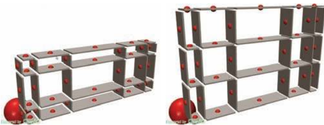
Figure 19: Presentation layout: Parametric shelf. All the boxes can be dragged to adjust the spacing, and pushing the red spheres inserts a new row or column of planks.
