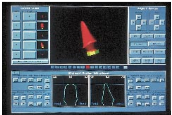
Figure 4: Procera CAD-CAM design image.
