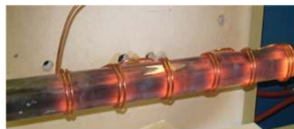
Fig. 4. A (left) drawing and (right) photograph of the six-coil array is shown during operation with a germanium-loaded graphite boat moving slowly through the series of RF coils. The bright regions in the drawing depict the regions of melted germanium.
