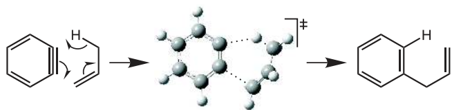
Scheme 3: Ene -type [4+2] cycloaddition in presence of an allylic hydrogen in the alkene component. Formation of the open chain, terminal alkene product for the reaction o -benzyne + propene.
