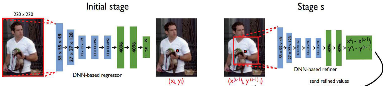
FIGURE 8. DeepPose's DNN-based pose regressor and refiner.
