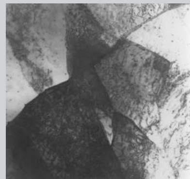
Figure 8. A photomicrograph showing the pinning of grain boundaries by dislocations.
