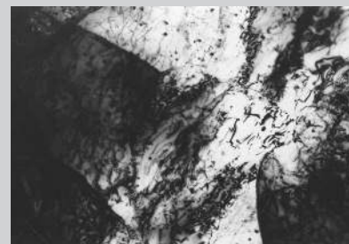
Figure 9. A TEM micrograph of Al-2.5Mg-0.5Sc alloy showing a high dislocation density at the sub-grain boundaries.
