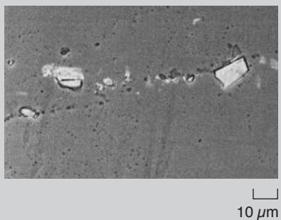
Figure 7. A SEM micrograph showing rectangular precipitates enriched in Ti, Al, and Sc.
