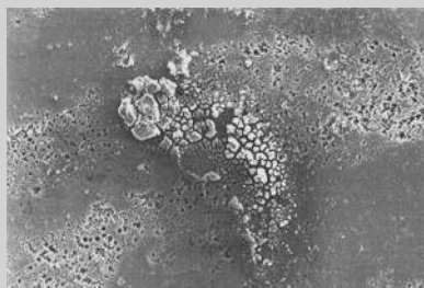
Figure 11. The formation of gelatinous \text{Al}(\text{OH})_3 in the form of mothballs and its cracking.
