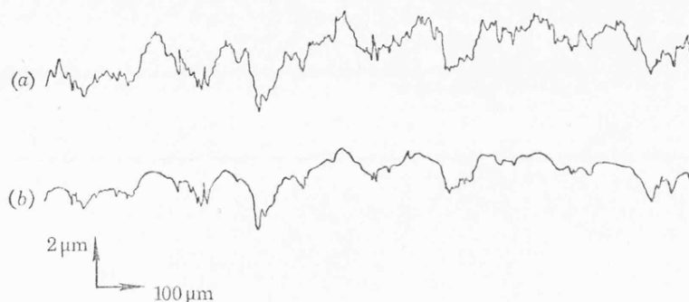
FIGURE 14. Talysurf profiles of cylindrical specimens used in lubricated friction experiments. (a) Original surface profile; (b) profile of the same line after one traversal of the load. Specimens 0.5% C steel; 300 d.p.n.; 0.035 mm diameter; load 25 N.
