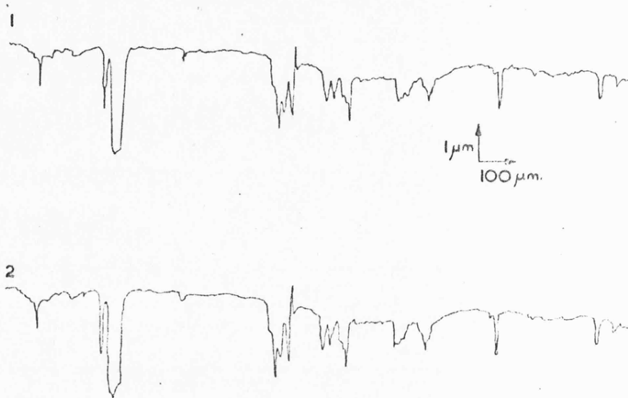
RECORDS 1 AND 2 TAKEN ALONG SAME TRACK, RELOCATING SPECIMEN AND READJUSTING MICROMETER BETWEEN TRACKS.
