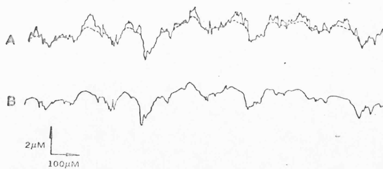
FIG. 11 TALYSURF PROFILES OF CYLINDRICAL SPECIMENS USED IN LUBRICATED FRICTION EXPERIMENTS. (A) Original surface profile (with profile of (b) superposed). (B) Profile of the same line after one traversal of the load. Specimens 0.5% C. steel, 300 D.P.N., 0.635 mm diameter, 32 \times 10^{-6} in. Load 2.5 Kg.
