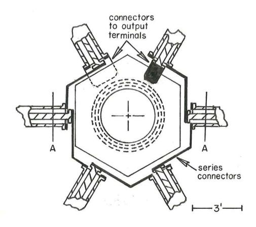
Fig. 5c. Detail of output terminal connections for series arrangement (section A-A from fig. 5b)
