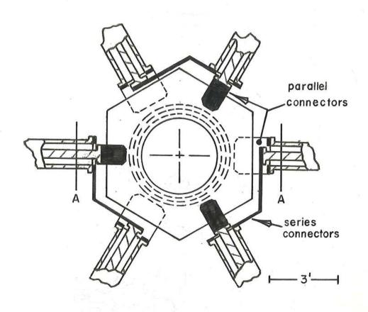
Fig. 5d. Detail of output terminal connections for series-parallel arrangement (section A-A from fig. 5b)
