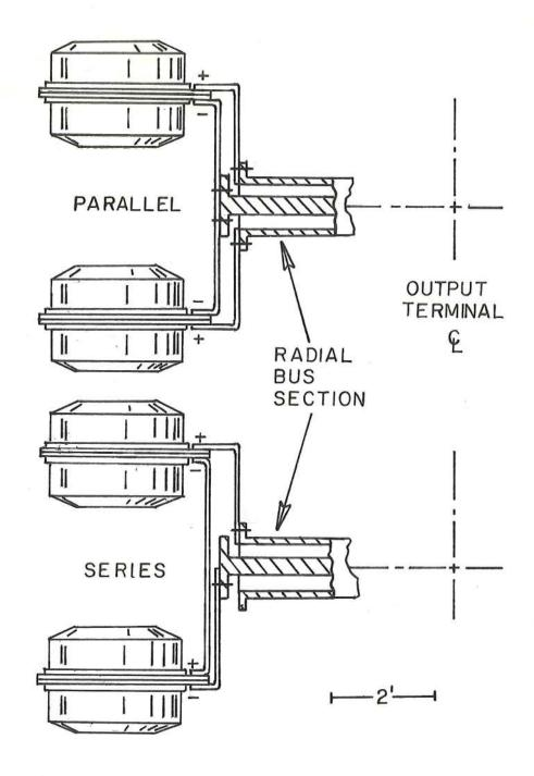
Fig. 5a. Detail of radial bus section connection at modular pair
