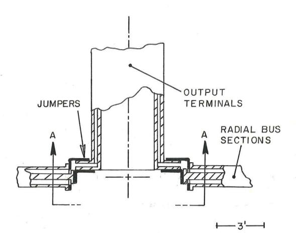
Fig. 5b. Detail of output terminal connections for parallel arrangement
