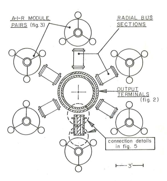
Fig. 4. Diagram of proposed HPG modular pairs surrounding central output terminals
