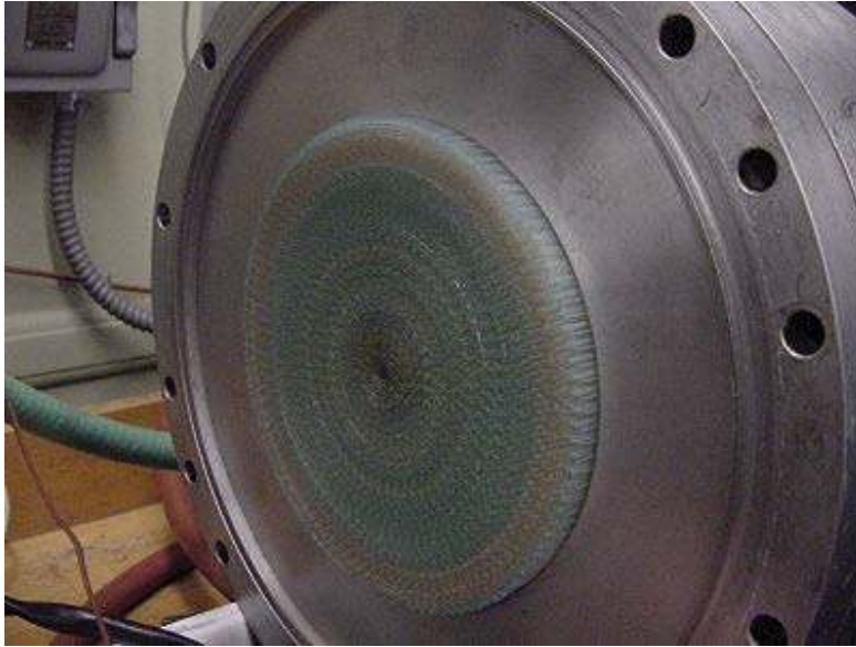
Figure 9. A Thermoacoustic Stack of Glass Tubing (Wikipedia).
