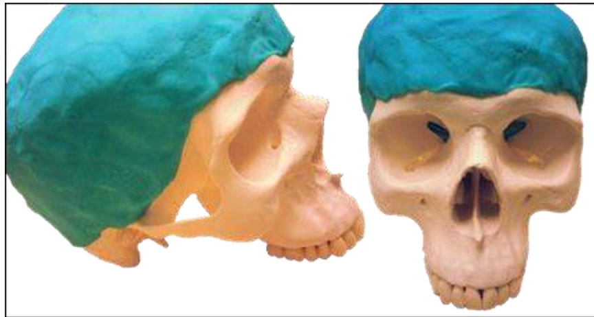
Figure 2.1. Synthetic three-shell realistic head model consisting of electroconductive dough which lines the inner and outer surfaces of a replica human skull. Lateral (left), rostral (right) views of the model showing the scalp layer.
