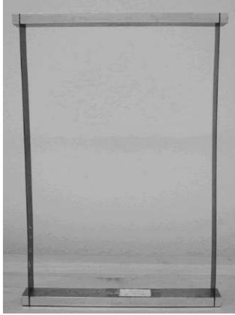
Figure 6.4: Photograph of the Parallel A(Steel) configuration of the mechanism.
