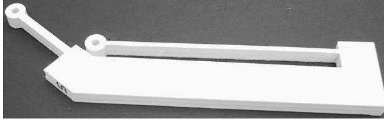
Figure 6.9: Number 5 test specimen for testing the dynamics of macro compliant mechanisms.
