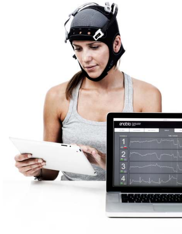
Figure 1.1: An example of an ambulatory psychophysiological set-up with an EEG amplifier plus mobile and fixed devices. Image reproduced with permission from Neuroelectronics SLU (Barcelona, Spain).
