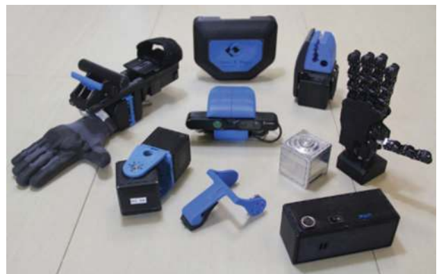
Figure 1. A set of components (grippers, compliant actuators, and batteries, among others) of the NMMI platform. Through them, flexible-joint robots can be intuitively built and tested.
