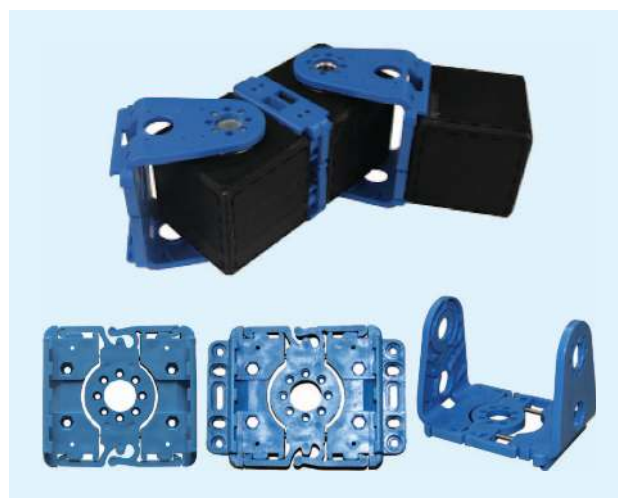
Figure 7. With the use of interconnection flanges (blue objects), rigid connection or revolute joints can be intuitively formed, obtaining more complex systems.
