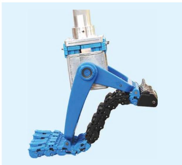
Figure 5. The Pisa/IIT SoftFoot is a passive deformable foot designed to adapt to uncertainties and walk on uneven terrain.
