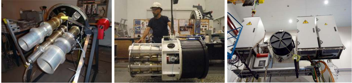
Figure 4. Left: Close view of the MFI, during the integration phase (May 2011). Center: Integration of the MFI in the QT1 focal plane (December 2011). Right: MFI already installed at the QT1 focal plane (January 2012). The electronic boxes controlling the telescope and the instrument are also installed.
