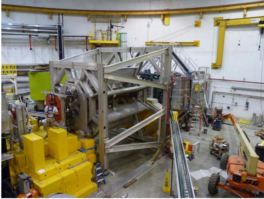
Fig. 2. The Q_{\text{weak}} experimental apparatus during installation, before most of the equipment was covered with shielding. The target scattering chamber is on the left, followed by the first two lead collimators on either side of the man in the figure. A third lead collimator faced with aluminum sits just in front of the large frame in the center of the picture, which supports the eight magnet coils. Three of the eight quartz detector bars appear just downstream and to the right of the magnet as skinny, long bars.
