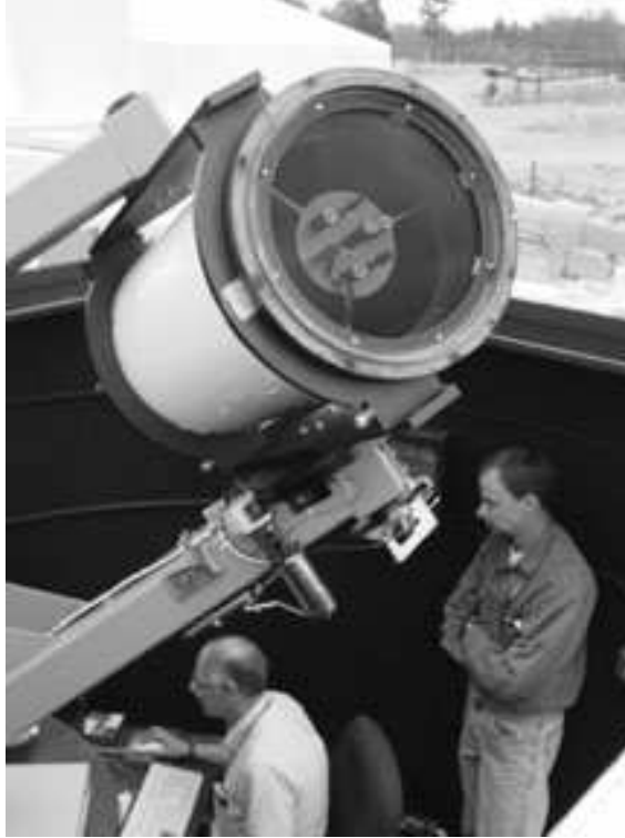
Figure 2. The RAPTOR-S telescope at Fenton Hill Observatory. It is a 0.3-m Ritchey-Chretien telescope with a low resolution spectrograph that responds in seconds to real time alerts generated by the wide-field sky monitoring system.
