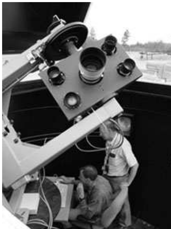
Figure 1. The RAPTOR-A telescope array which is part of the stereoscopic wide-field monitoring system. The four wide-field imaging cameras surround a central fovea telescope and the entire array is mounted on a rapidly slewing robotic mount. The telescope is housed in a robotic enclosure and is designed to run in a fully autonomous manner.
