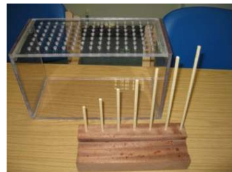
FIG. 3. Thickness measuring device (TMD) and rods.
