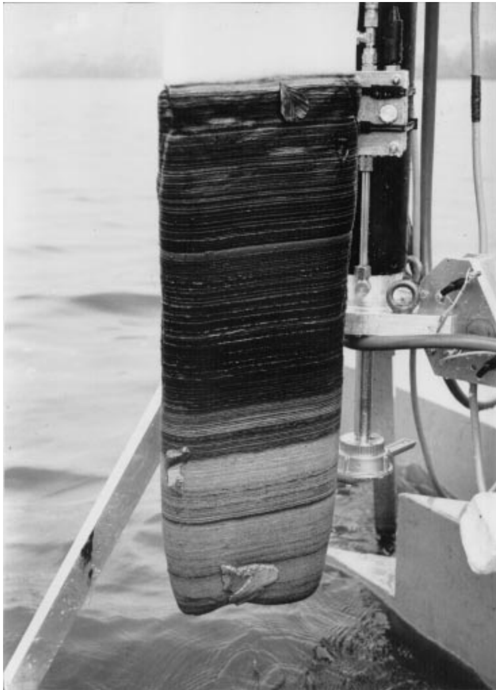
Figure 2 Freeze-core taken in the deepest part of Baldeggersee at 66 m of water depth. The water/sediment interface represents autumn 1993.
