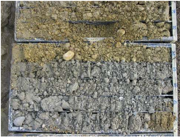
Figure 9. Gravel core from 23 to 30 m depth from borehole SPB-3 – test field GW (Đurđevac) (see Fig. 10a).
