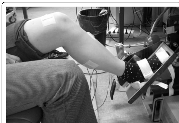
Figure 1 Measurement set-up. The subject's ankle was fixed on the footplate that was rotated by an electrically powered single axis actuator. Ankle reaction torque, ankle angle and EMG were measured during imposed ramp-and-hold movements.
