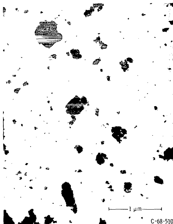
Figure 4. - Transmission electron photomicrograph of chromium powder after ball milling in water for 768 hours.
