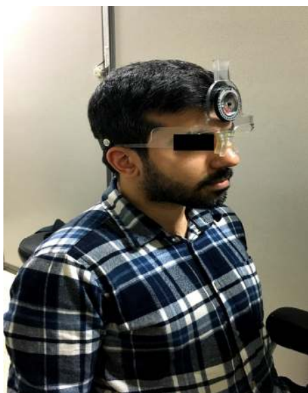
Iranian Rehabilitation Journal Figure 1. The measurement of cervical rotation with CROM device, while the subject sat on the chair in a straight position
