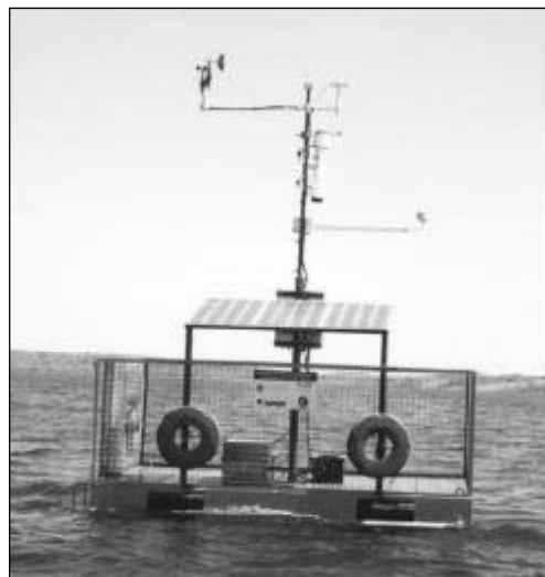
Fig. 2 — The SMATER unit consisting of a climatological station, a solar panel a data logger and a YELLOW SPRINGS 6.600 sensor (original IIE).
