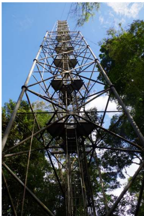
Fig. 3 The 55-m high eddy flux tower set up in 2003 in French Guiana (Bonal et al. 2008) (credits D. Bonal). Equipment installed on top of the tower (above the canopy) allows to continuously monitor the gas exchange ( \text{CO}_2 , \text{H}_2\text{O} ) between the atmosphere and the considered ecosystem (around 50–100 ha)
