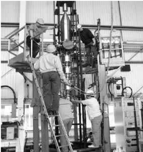
Figure 2: Marconi 402.5 MHz, 2.5 MW pulsed klystron.
