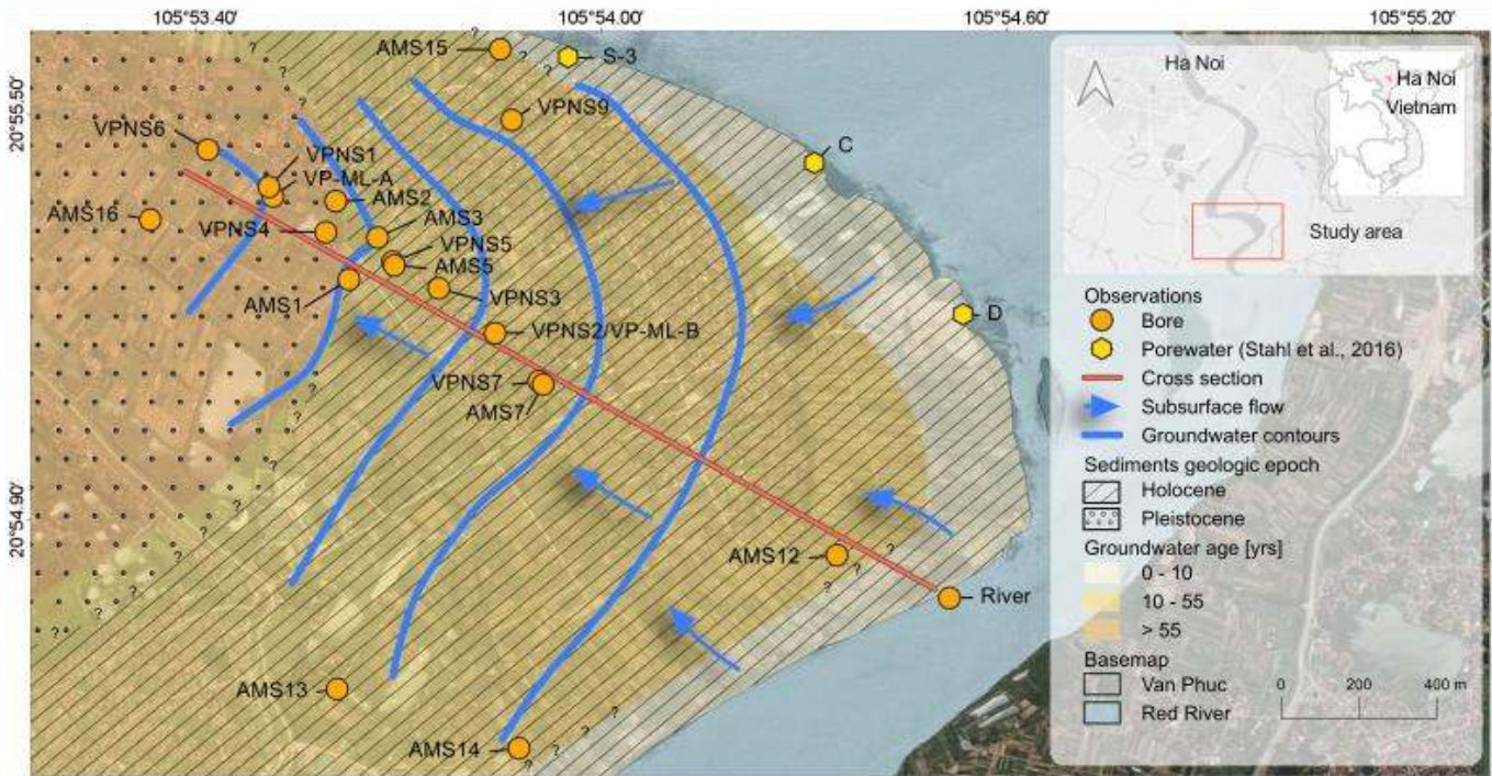
2 Fig. 1: Field site, observation bores and approximate distribution of Holocene and 3 Pleistocene sediments in the study area (reproduced after van Geen et al., 2013 7 ). Water 4 level contours assessed on the basis of hydraulic heads (head data from November 2006 5 and June 2010) and main groundwater flow direction; groundwater ages inferred from 3 H– 6 3 He Tri concentration data. Orange line: Location of modelled cross section.
