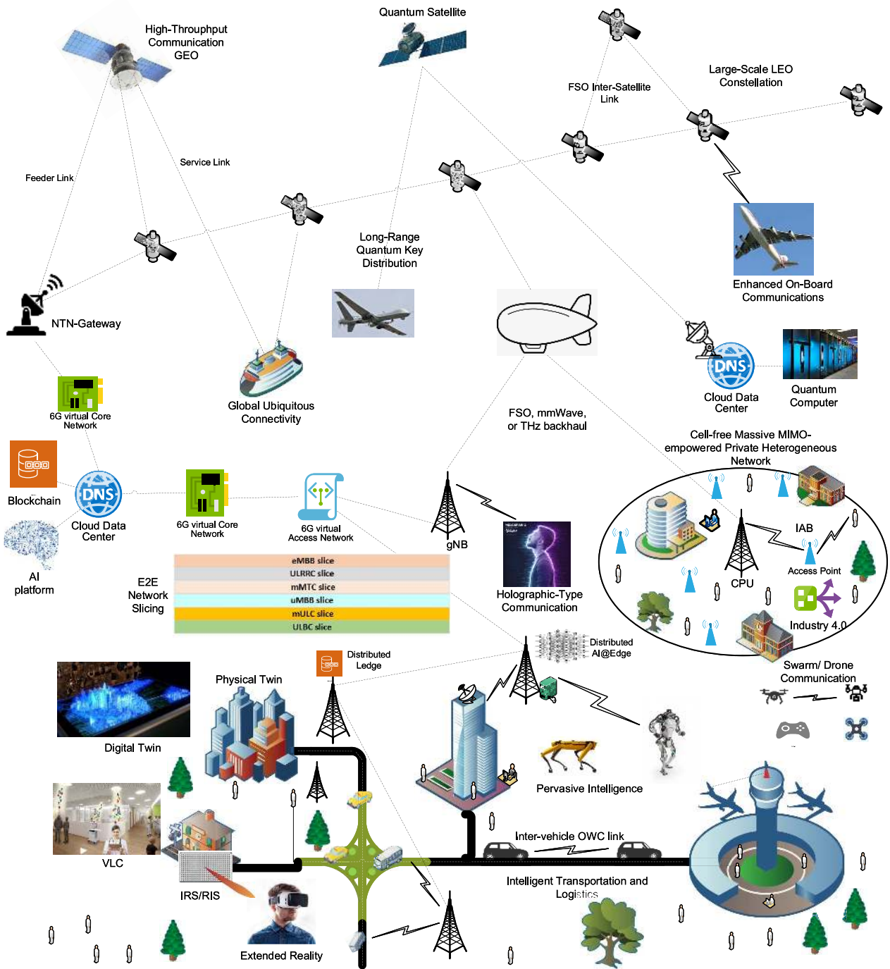
FIGURE 3. Envision of the deployment scenarios and architecture for 6G, demonstrating representative use cases and some of key technological enablers.
