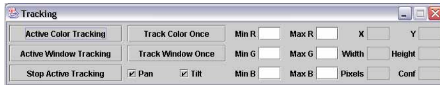
Figure 11: The CMUcam Tracking window enables iPAQ visual tracking code to be launched
