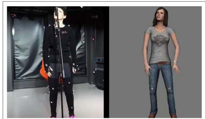
FIGURE 7 | Body motion capture via OptiTrack motion capture system (Opt, 2020) and the corresponding mapping to one of the Microsoft Rocketbox avatars in a singing experiment by Steed et al. (2016a).
