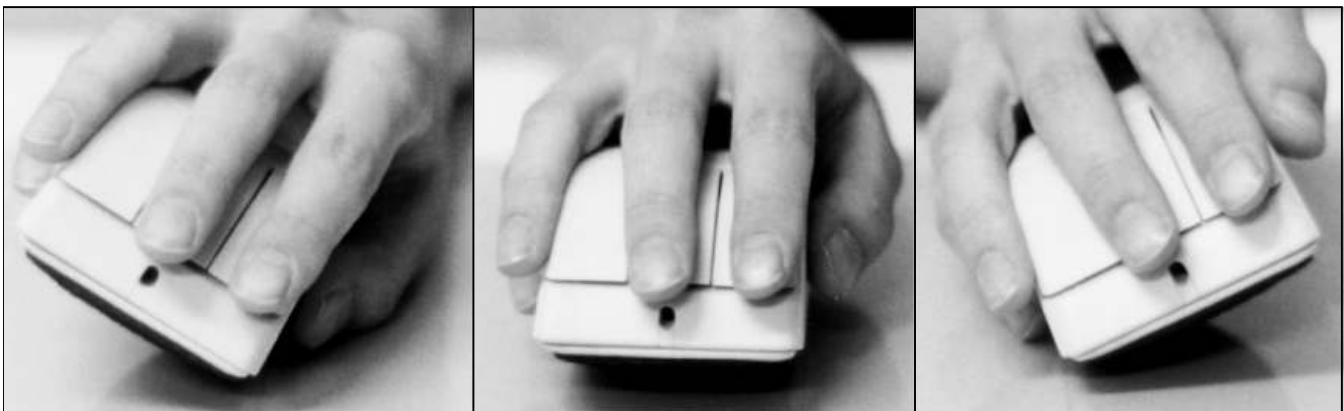
Figure 2. Tilting action of the Rockin’Mouse
