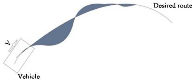
Figure 9. Lateral displacement area.
