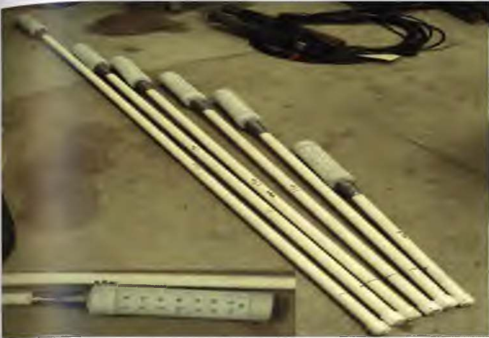
Plate 4.7: Piezometers and close up of piezometer tip (filter section)
