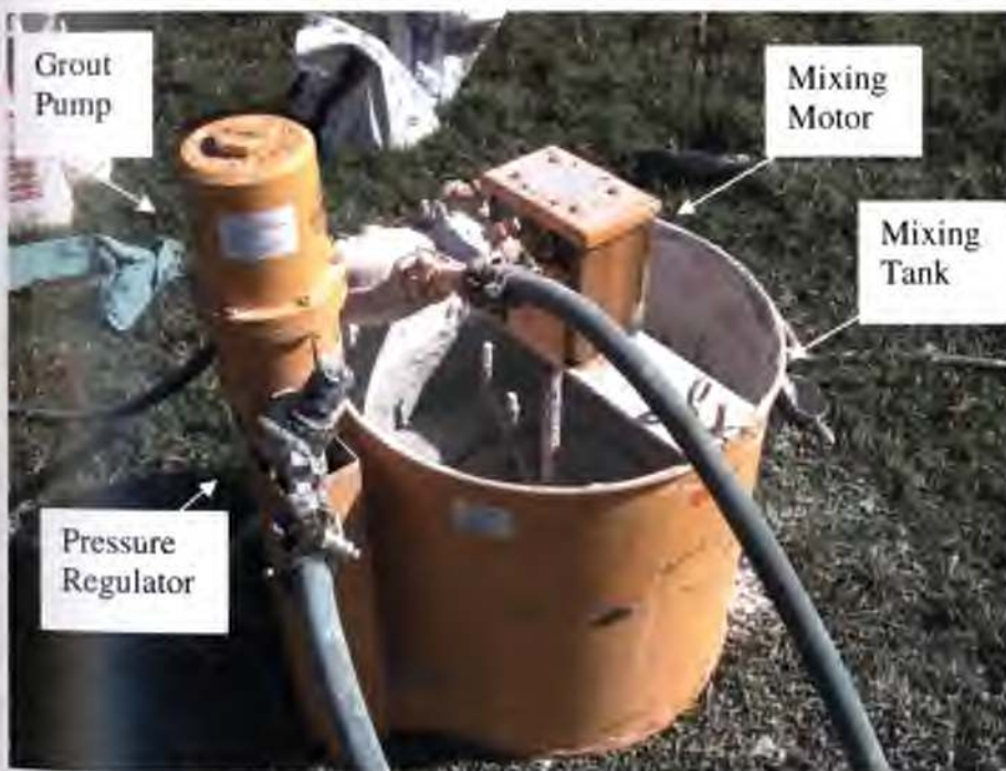
Plate 5.1: Injection equipment including Mixing tank, grout pump, mixing motor and pressure regulator.
