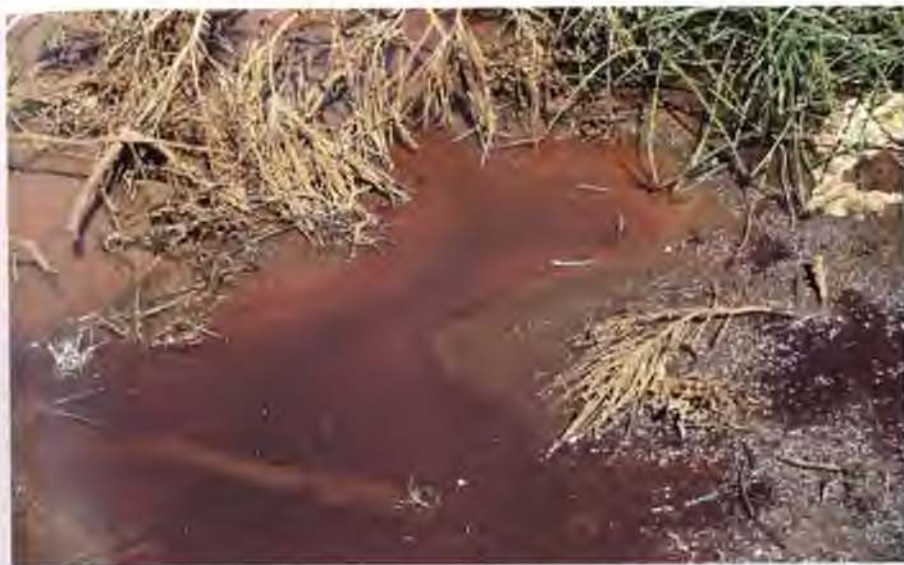
Plate 7.1: Iron oxide flocculation in flood mitigation drain adjacent to lime-fly ash barrier study site.
