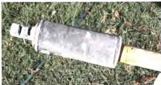
Plate 5.3: Modified tip of injection pipe.
