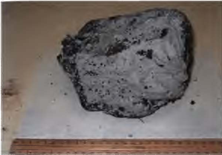
Plate 5.6: Excavated section of barrier (from preliminary injections)
