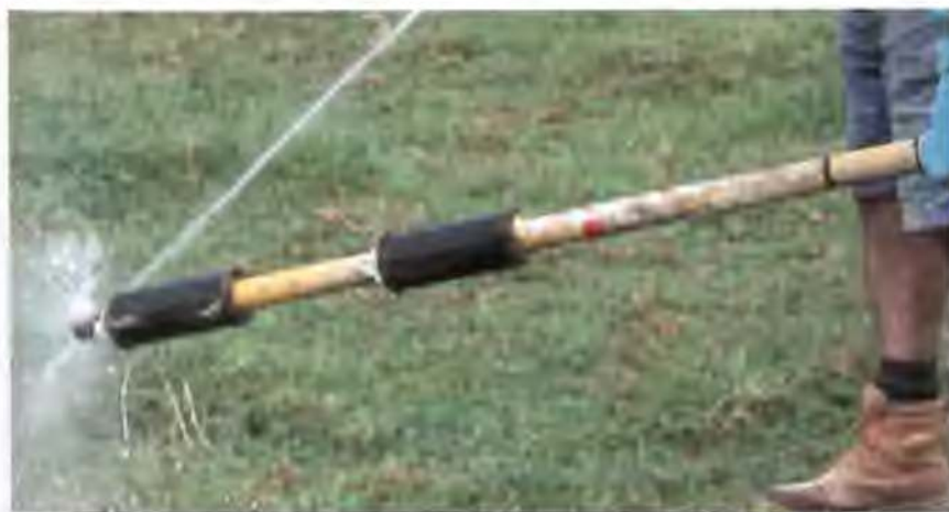
Plate 5.4: Modified design of injection pipe. Note the two sets of packers.
