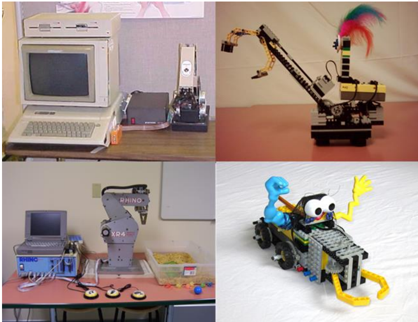
Figure 1 Robots used in reported studies. Clockwise from top left: MiniMover, Lego Minstroms Arm, Lego Roverbot car, Rhino.
