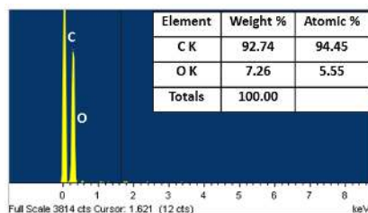
Figure 4. EDX spectrum of the MWCNTs oxidized with \text{H}_2\text{SO}_4/\text{HNO}_3 mixture for 6h at 100^\circ\text{C} ; inset is the table showing the percentage of each component in the nanotubes.
