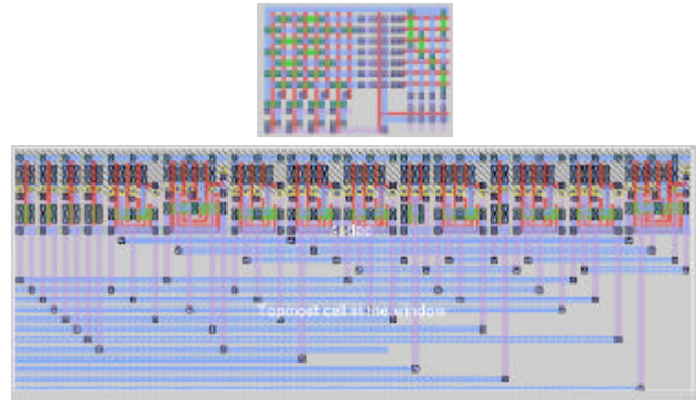
Figure 4: Comparison of standard-cell and PLA layout for a simple 4-input 4-output logic function
