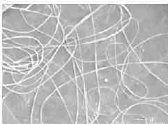
Fig. 2. Examples of biocompatible PEO (a), biodegradable PLGA (b), and natural collagen (c) nanofibers produced by electrospinning.
