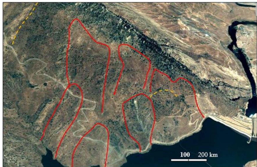
Fig. 5 Interpreted satellite image near Derbendikhan Dam showing unstable slopes in red lines and dashed orange lines shows cliffs (after Sissakian et al. 2019)
